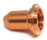
The 0.65 mm short nozzle for PT60 torches is ideal for precise cuts in the 10 to 20 amp range. Its compact design allows superior control in tight spaces and detailed work. Made from highconductivity materials, it ensures arc stability and greater durability. Compatible with plasma cutting processes, it offers an excellent balance between performance and precision. Includes 2 units.
