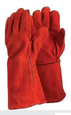
The PRO SOLTER Welding Glove is the best choice for welders seeking thermal protection, durability, and comfort in their daily work. Made of split cowhide leather, it features reinforced Kevlarstitched seams and a soft inner lining offering maximum resistance to heat, sparks, and abrasion Its ergonomic and flexible design ensures a firm grip without compromising safety. Ideal for MIG/MAG, TIG, and MMA welding, handling hot metals, and industrial work. Protect your hands with Solter's quality!
